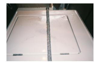
6 Month inspection shows continued deterioration of the anode rod.
